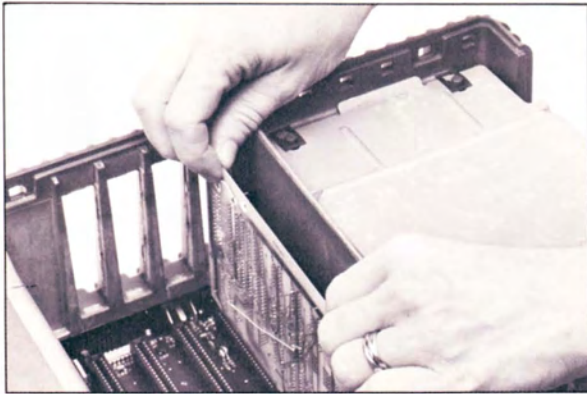
Figure 2-4. Installing the Interface Card
