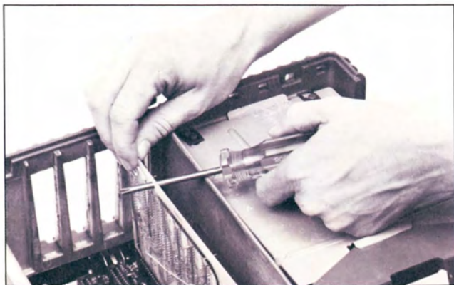
Figure 2-3. Removing a Dummy or a Peripheral Card
